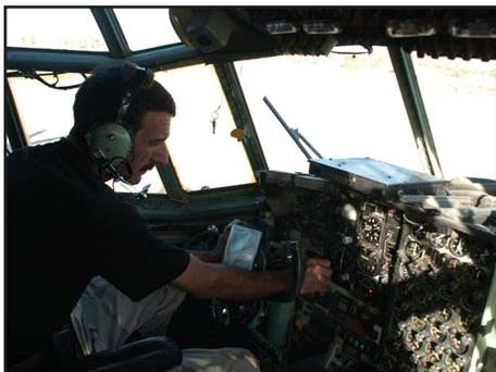
**An Iraqi airman performs a pre-flight inspection on a C-130E aircraft at New Al Muthanna Air Base, Sept. 19. The Iraqi Air Force currently has three C-130Es, and expects to receive another three by 2008.**
